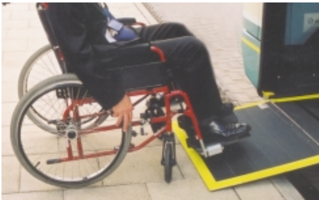
The operation of wheel chair boarding and other disabled access features will be checked at annual test
