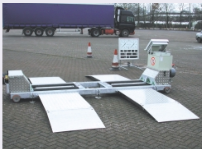
Mobile Roller Brake tester – improving enforcement at the roadside
